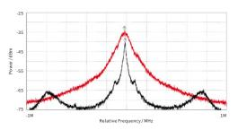
Spectrogram of beat between an ECDL and a fiber laser with (black) and without (red) external PID-lock of the ECDL to the LWA-1k confirming the lineshape spectrum in the graph to left.
