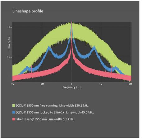
The LWA-1k featuring an improved resolution enables the analyzation of laser with very narrow linewidths down to 2 kHz. The analyzer unit automatically generates an output signal that is evaluated by the digitizer unit, connected to a PC via USB. An intuitively usable software interface performing the analysis provides the frequency noise related plots and values, such as the frequency noise spectrum and the lineshape spectrum together with the results of intrinsic and combined linewidth.
